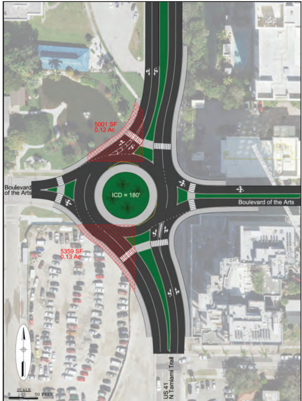
One of the four different roundabout alternatives evaluated at this intersection. To make this a feasible alternative, additional right-of-way access is needed.
